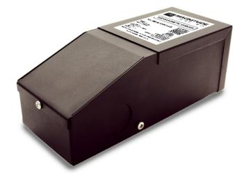
Magnitude's M60L12DC-AR is the most compact LED driver on the market with a magnetic transformer core. It is equipped with two auto-reset breakers, one on the input and one on the output, which protect both the load and driver. The driver is encased in a coated metal box that includes 2 knock-outs, one on each side, to enable easy installation that complies with electrical code requirements.
