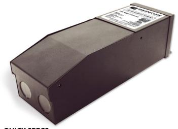
Magnitude's M100L12DC-AR is the most compact LED driver on the market with a magnetic transformer core. It is equipped with two auto-reset breakers, one on the input and one on the output, which protect both the load and driver. The driver is encased in a coated metal box that includes 2 knock-outs, to enable easy installation that complies with electrical code requirements.
