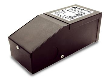
Magnitude's M40L12DC-AR is the most compact LED driver on the market with a magnetic transformer core. It is equipped with two auto-reset breakers, one on the input and one on the output, which protect both the load and driver. The driver is encased in a coated metal box that includes 2 knock-outs, one on each side, to enable easy installation that complies with electrical code requirements.
