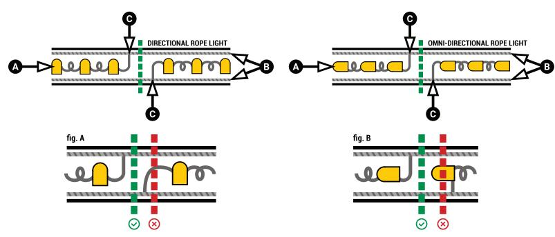
To safely cut your rope lights without a cut mark or to confirm if a cut mark is correctly placed locate and identify each of the following components:
