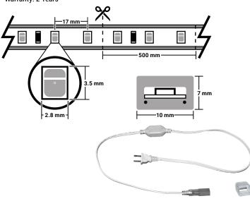
120V Strip Light Power Cord & End Cap pre-installed on all spools and custom cuts
