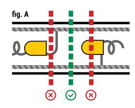
To safely cut your rope lights without a cut mark or to confirm if a cut mark is correctly placed locate and identify each of the following components:
